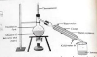
water condenser, and a Bunsen burner. The apparatus is arranged as shown in the above figure. Then, the mixture is heated slowly. The thermometer should be watched simultaneously. Kerosene will vaporize and condense in the water condenser. The condensed kerosene is collected from the condenser outlet, whereas petrol is left behind in the distillation flask.
